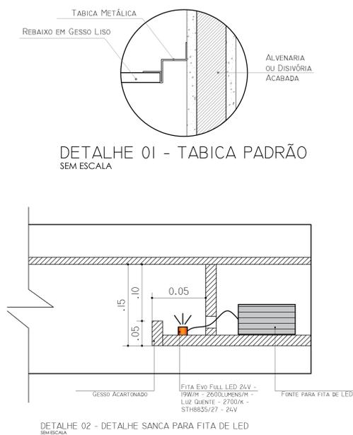
DETALHE 02 - DETALHE SANCA PARA FITA DE LED SEM ESCALA
